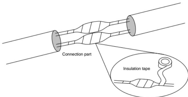
2. Waterproof the cables with self-adhesive waterproof tape.
