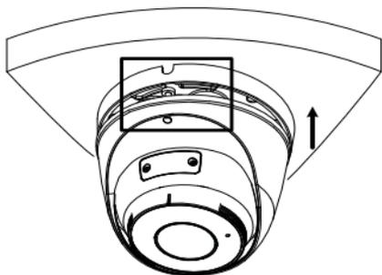
Adjust the housing to the position shown in figure above. Align the screw hole on the
