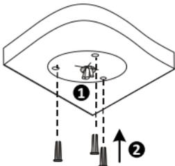
3. Loosen the fixing screw, then remove the housing. Loosen the fixing screw, then turn the housing to the position shown in figure ❶ to remove it.
