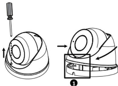
4. Connect the cable and then secure the bottom ring.
